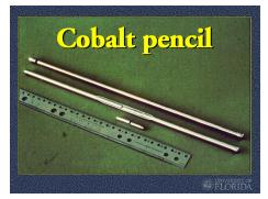
These pellets are then placed in "pencils" that are about 3/8's of an inch thick and 15 inches in length. However, before they can be useful to pasteurize or sterilize products, the cobalt must be made into a radioactive form. Commonly, , these pencils of cobalt are used as control rods in existing nuclear power plants, and as a consequence, become radioactive. Cobalt is mined; it is waste produced by nuclear industries.
