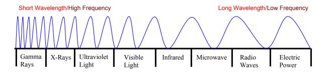
Radiation is called **ionising** radiation when it is at a sufficiently high frequency (gamma rays and X-rays) that it results in the production of charged particles (ions) in the material that it comes in contact with. **Non-ionising** radiation, such as that from microwaves, does not produce ions but can create heat under moist conditions and is routinely used for purposes such as cooking and re-heating of foods.
